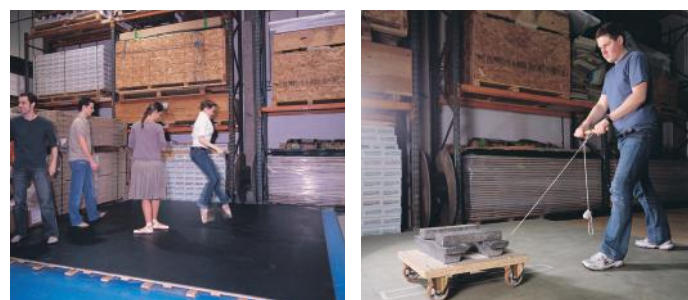
The photos show tests to DIN 18032-2 in progress on Harlequin's WoodSpring basket weave floor with Harlequin Cascade surface and dancers from The Royal Ballet, London, approving the test floor.
